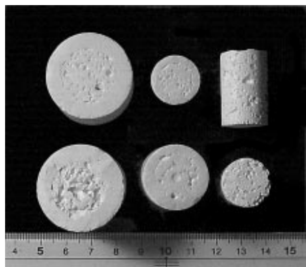
Figure 5 Cross-sections of cement/foam cement composites of different sizes and foam cement cores only.
